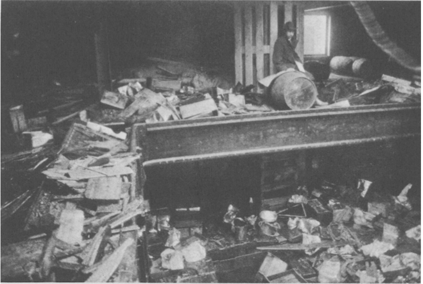
Wreckage after discharge of vegetable oil cargo at San Francisco in 1920, resulting in 4 feet of oil leakage in bilge of this hold.
