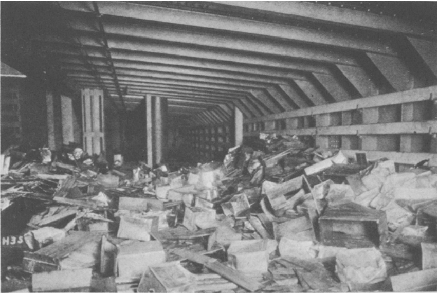
Another view of same vessel as photograph above, showing result of poor stowage and rough weather
